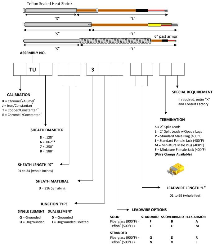
\*.062 Diameter Tube uses only 30 AWG solid PFA Teflon<sup>®</sup> or Fiberglass wire. Available in single junction only.
