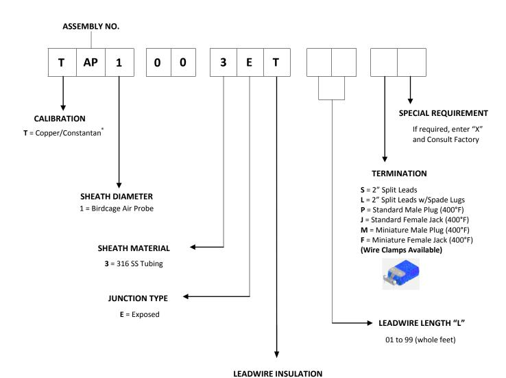
T = 22 AWG Stranded FEP Teflon® (-196°C -200 °C) Freezers / LN2
