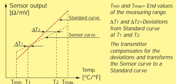
**System error correction** -This method is used to correct the system error (sensor + transmitter error) by exposing the sensor to one (one-point correction) or two (two-point correction) accurately measured temperatures (true temperatures). The true temperature(s) and the corresponding transmitter reading(s) are entered, and the transmitter automatically corrects for the system errors. *Fig. 3.*
